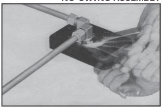
When assembling into a LDI Port, the fitting remains stationary. Only the swivel nut turns
